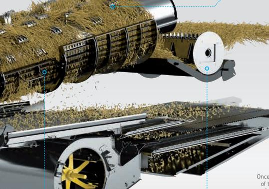
Once the straw has reached the end of the rotors, the 400mm diameter straw flow beater moves straw onto the positive straw discharge belt. This belt directs the straw rearwards, for efficient flow through to the rear of the combine.
